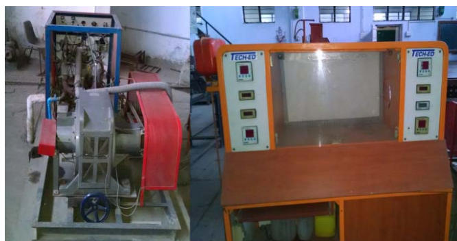
Fig. 4: Photograph of computer controlled 4 stroke 4 cylinder MPFI petrol engine test rig with control panel.
